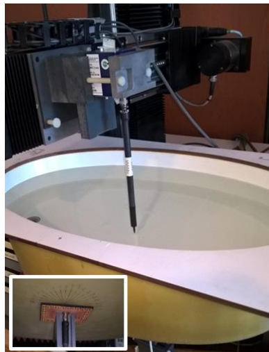
Fig. 14: SAR assessment setup consisting of the standardized flat phantom, dosimetric probe, automated positioning system, and ATTO cell antenna positioned below the flat phantom (inset).
